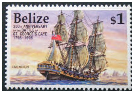
Fig. 1. His Majesty's Sloop MERLIN. Built by John Dudman, Deptford; launched 25 March 1796. Broken up at Deptford in January 1803. Dimensions & tons: 106ft x 28ft x 13ft 9in. 365 tons. Men: 121. Guns: Upper Deck 16 x 6 pounders; Quarterdeck 4 x 12 pounder carronades; Forecastle 2 x 12 pounder carronades. Commemorative stamp, Belize, 1998. (© Belize Post Office Department)
