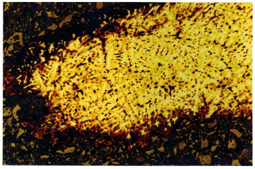
$$\operatorname{Fig.}\ 6$$  #R1560, general view of cast structure, etched, x125
