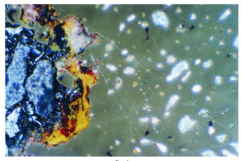
FIG.~4 #R1560, as Fig. 3 but viewed under plane polarised light; cuprite-rich corrosion is red/yellow, lead corrosion products are white, and lead metal is mottled grey, unetched, x625
