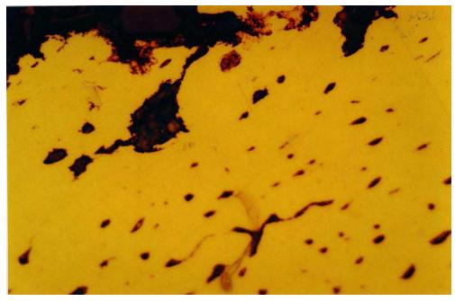
$$\operatorname{Fig.} 5$$  #R1560, another area; elongation of lead inclusions indicate local deformation, unetched, x625
