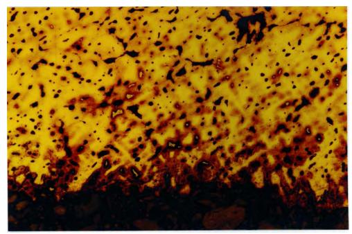
$$\operatorname{Fig.} 8$$  #R1560, the other, undeformed, surface, etched, x250
