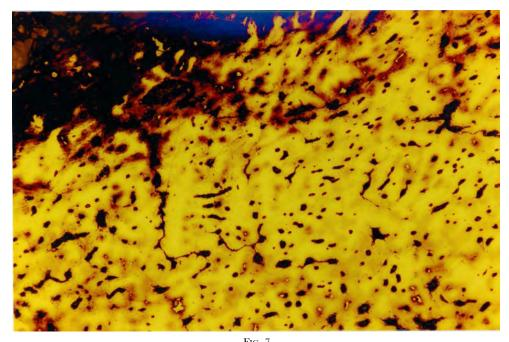
Fig. 7 #R1560, showing deformed part of sample with some deep intergranular corrosion (left of centre), etched, x250
