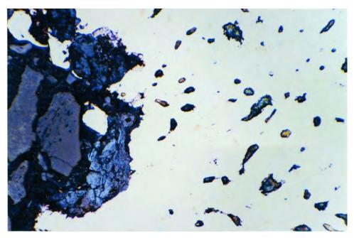
$${\rm Fig.}~3$$  #R1560, another area showing evidence of replacement of lead inclusions and build-up of corrosion products in surface pits, unetched, x625
