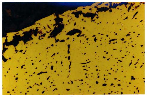
$$\operatorname{Fig.}\,1$$  #R1560, showing corrosion cavities beneath the surface with deeper intergranular corrosion and some intergranular corrosion; note also interdendritic lead distribution, unetched, x250
