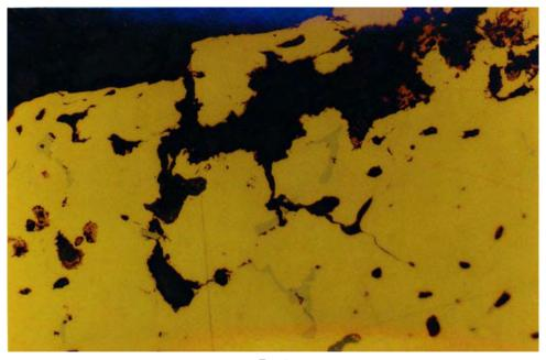
$$\operatorname{Fig.} 2$$  #R1560, detail of corrosion showing formation of redeposited copper, removal of lead, corrosion at phase boundaries, and possible de-alloying, unetched, x625
