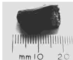
FIG. 29 Drawn iron wire rivet from Braunton, Devon
